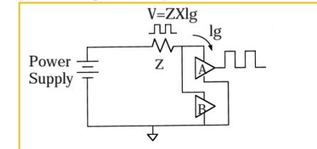
Thus, a noise voltage is developed across this impedance. A high frequency, noise voltage that will have the same spectral content as the switched gate.
