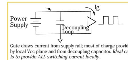
The problems occur when the plane is cut and some impedance is inserted in series with the plane. Sometimes a ferrite bead is used, sometimes an inductor is used and sometimes the plane is reduced to a small interconnect trace.
