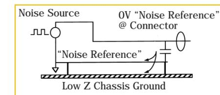
Signal control: stopping noise at its source
